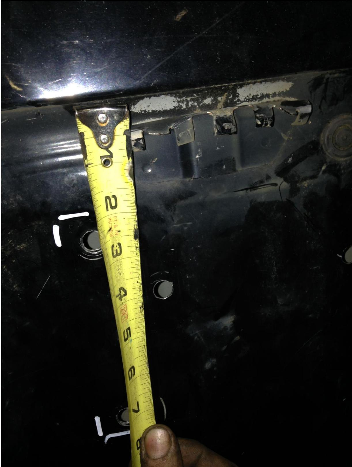
b. drill the two marked holes with the 7/16" drill bit and bolt the inner structural panel to the *outside* of the vehicle.
