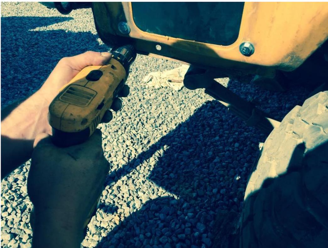
(4) Place structural inner panel into pocket between inner and outer body sheet metal through the access hole in the rear hatch. Make sure the two welded nuts are facing down. Loosely place 2 bolts with washers through the holes drilled in the sheet metal of the truck and thread them into the nuts welded to the structural inner panel.
