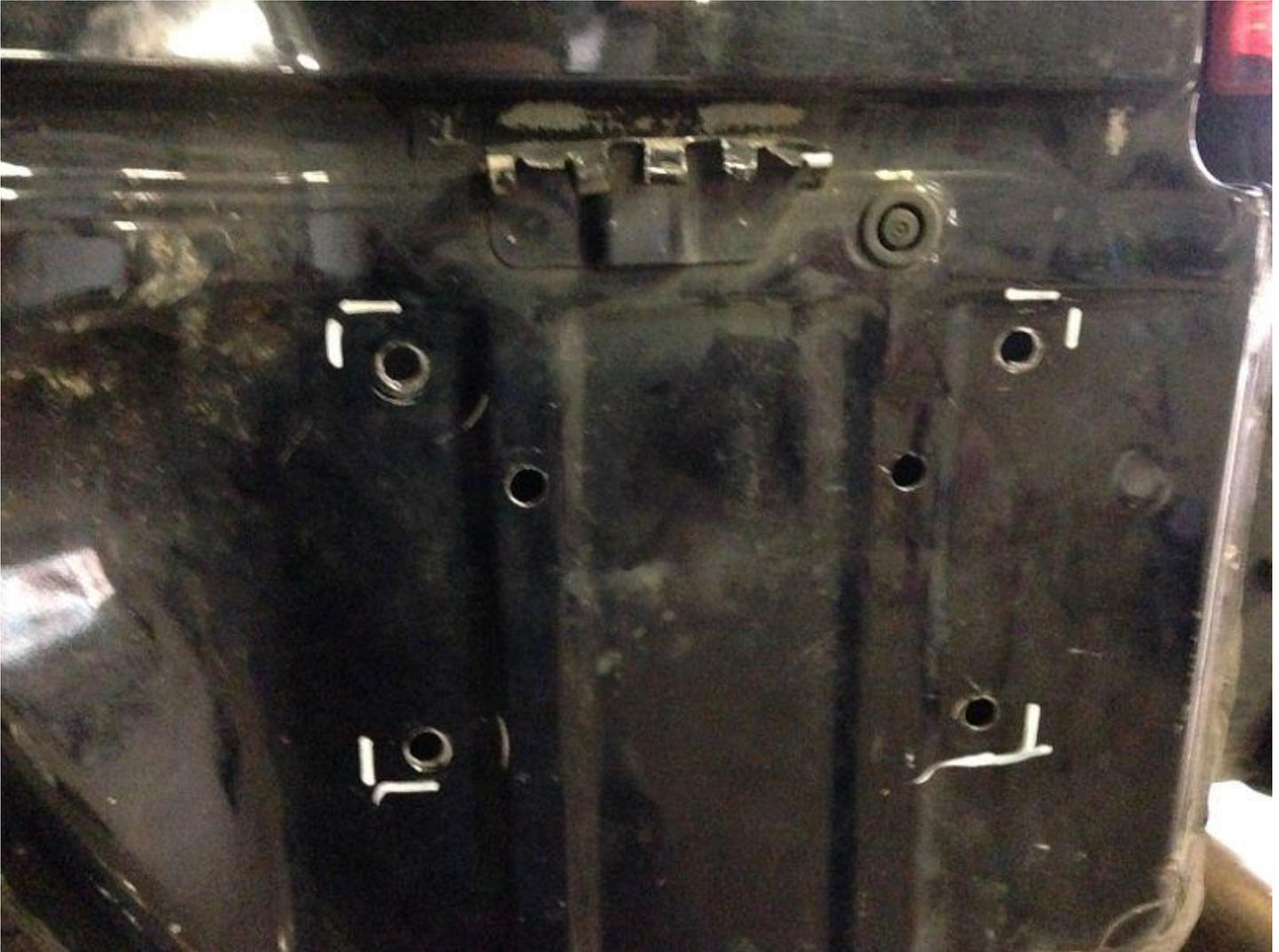
e. Drill holes in lower pinch seam that originally held plastic corner retaining bracket to 7/16"
