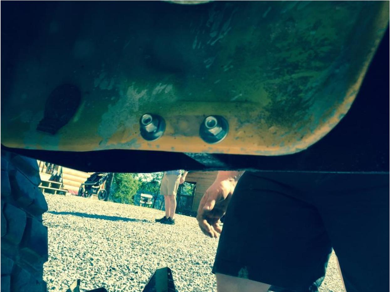
OE Plastic corner should now pull off vehicle from the tabs located under the tail light and along the top side panel.
