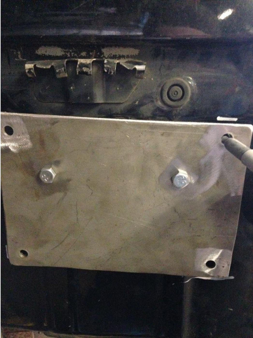
c. mark the 4 corner holes through the inner structural panel onto the sheet metal of the vehicle as shown in the figure above.
