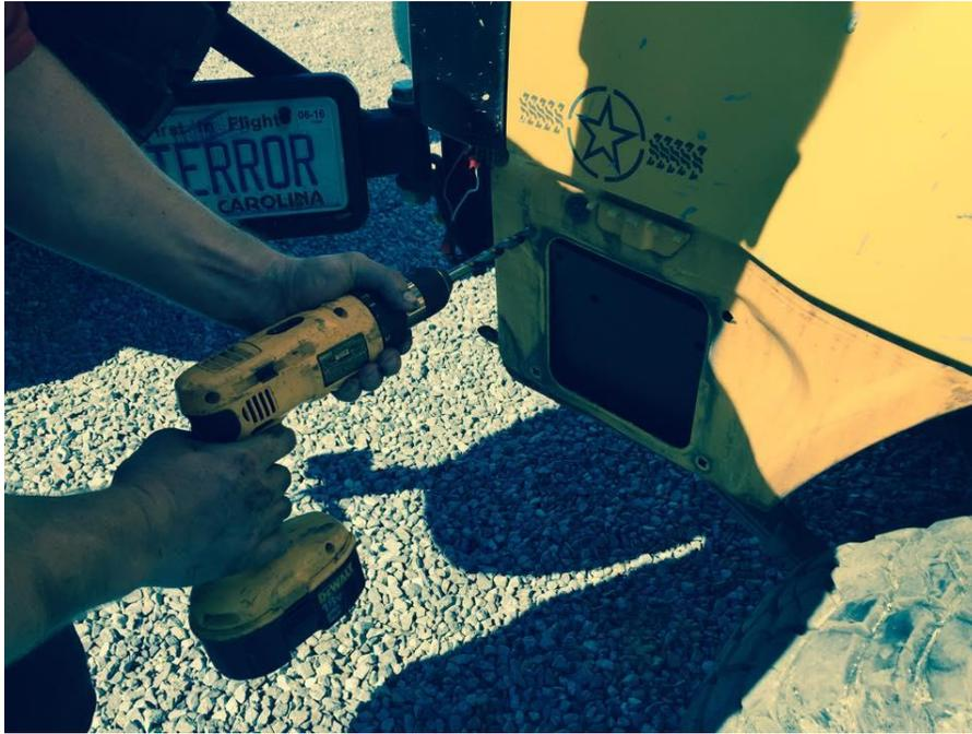
d. Drill the 2 holes out on the pinch seam that held the original corner support bracket using a 7/16” drill bit.
